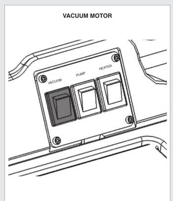
Turn on vacuum motor and begin cleaning. For best results make two dry passes to every wet pass.
