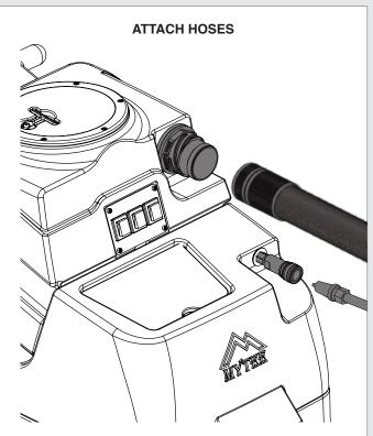
Attach one end of a solution hose to a wand or other tool, the other end to the Spyder's  $^{\text{TM}}$  front quick disconnect. Attach one end of a vacuum hose to the tool, the other end to the Spyder's  $^{\text{TM}}$  Cuff-Lynx  $^{\text{TM}}$  vacuum hose port.
