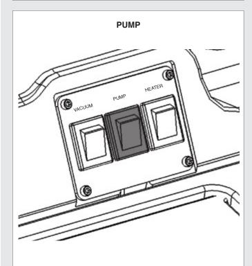
After the machine has been plugged into a 20 amp grounded outlet, turn on pump. Squeeze the trigger on the tool until it releases a steady flow.
