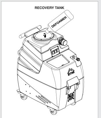
Add a defoamer in the recovery tank to reduce foam, prolonging the life of the Spyder  $^{\rm TM}$  vacuum motor .
